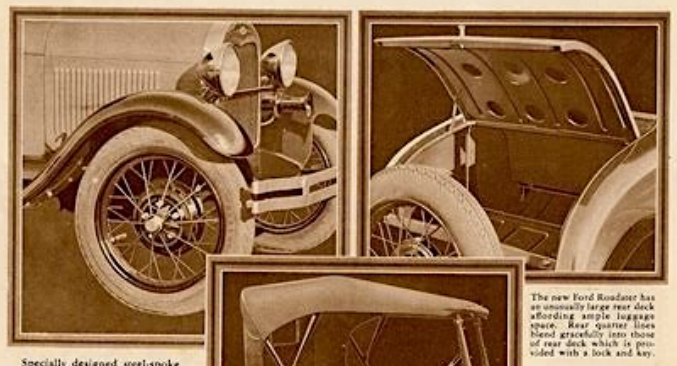
Specially designed steel-spoke wheels, standard on all types, help to emphasize the alert, fleet appearance of the new Ford Roadster. These steel-spoke wheels are welded in one piece, and there are only thirty spokes in each wheel.
