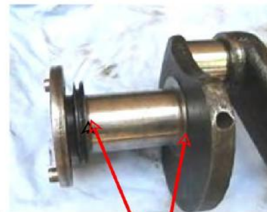
Crankshaft Rear Main Bearing Thrust Surfaces
