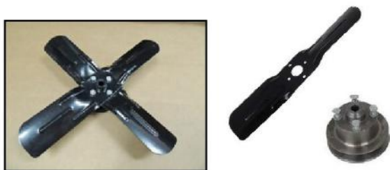
Poor quality replacement fans that use bolts to attach the blades to a steel or aluminum hub
