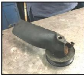
Original Model A fan that failed
