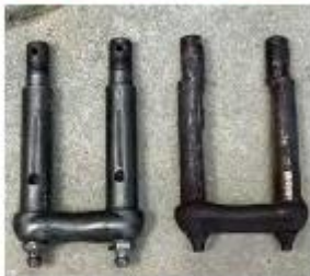
Side-by-side comparison to new shackle (left) and old (right)
