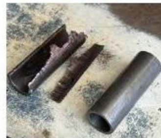
Worn spring bushing (left) with new (right)
