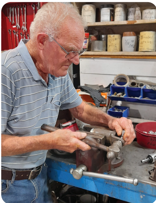
Gene Lucas removing the driveshaft bearing for Harry Brazier
