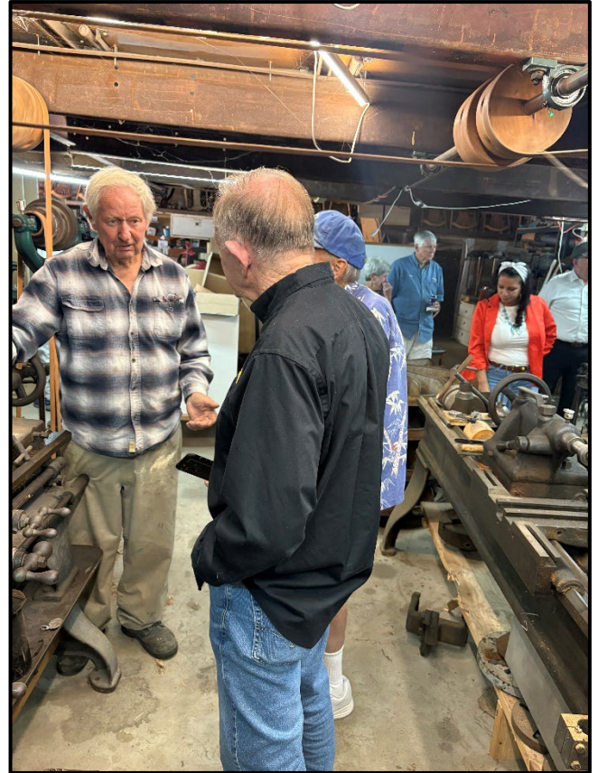
Dick Anderson explaining his belt pulley system for running the machines in his shop to Walt and Randy. What a treat to get a guided tour of the shop.
