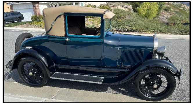
1928 Model A Sport Coupe Soft top with the lift up rear, Burtz engine, Mitchell Overdrive, V8 clutch and pressure plate, Brassworks touring radiator, Model B intake, carb, fan blade and oil fill tube, dash has water temperature and oil pressure gauges added, pop-out ignition switch, 6 volt negative ground, rebuilt shocks, LED lights, beautiful LeBaron Bonney interior, year of manufacture plates, Spartan ahooga horn and many other features. Call David at 818-825-9257 and see more photos at 1928FordModelA.com $27,750
