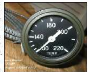
Mechanical temperature gauge with a 270 degree "sweep" dial
