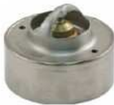
Thermostat for installation in the upper radiator hose
