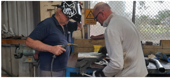
Pat Murphy teaching Geoff Tenbrink welding and fabricating a new expansion chamber for his motorbike
