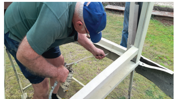
Pat Murphy injecting rust proofing into Jeff Cox's body frame
