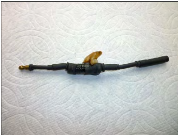
An ahooguh dropping resistor that burned out
