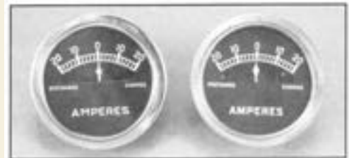
Two styles of lettering were used all years, see photo. Note the different styles of the ammeter pointers
