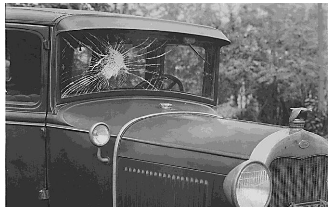
An example of Triplex Glass integrity in an original Model A
