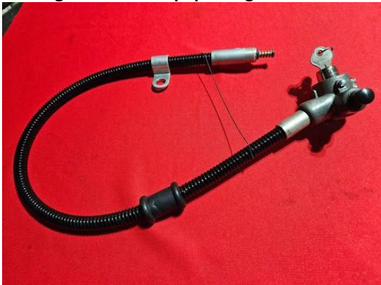
Same switch as above with armored flex cable
