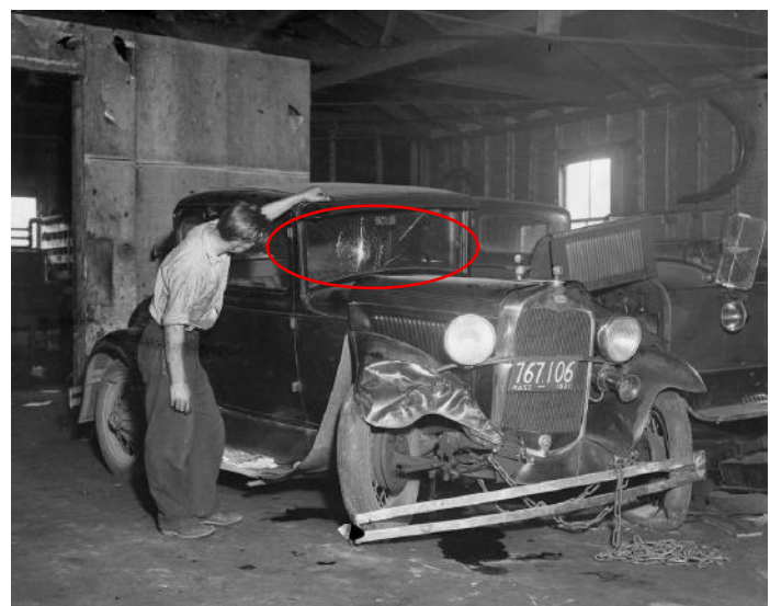
Passenger's head hit the windshield, Triplex held
