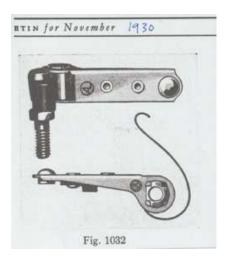
After experimenting with the first two methods, using a Dremel tool with a cut-off wheel, I cut the loop attaching the points to the mounting post like the method used by Larry and similar to the original points depicted in the Ford Service Bulletin (above).
