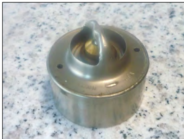
An automotive thermostat modified for use with a Model A. Note the skirt welded to the base to prevent it from tumbling in the water outlet hose. Two small holes are drilled into the base for a small amount of water flow when the thermostat is closed.
