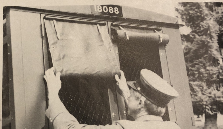
Above left: There are "dogcatcher" style screens instead of windows at the back. Above right: Tools and spare parts hide under driver's seat. Below left: Simple lock keeps the mail safe while in transit. Below right: Side curtains protect cargo from inclement weather.
