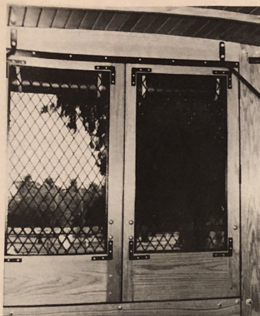
Above left: There are "dogcatcher" style screens instead of windows at the back. Above right: Tools and spare parts hide under driver's seat. Below left: Simple lock keeps the mail safe while in transit. Below right: Side curtains protect cargo from inclement weather.
