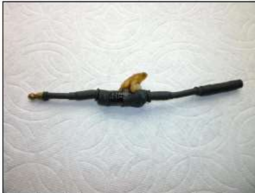
An ahooguh dropping resister that burned out
